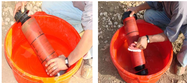
Fig. e: Cleaning of disc filter.
